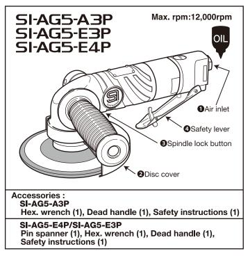
3. Pour approx. 0.5cc (2 to 3 drops) of the oil through the coupler. Connect it to the air hose, and run for 3 to 5 seconds to circulate the oil.
