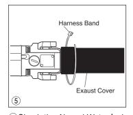
Sheck the Air and Water leak from the Hose connection. Put the Exhaust Cover on the tool and fix it by the Harness Band which enclosed in the box.
