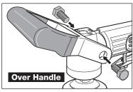
2. Firmly mount the pad so the spindle not to turn with the spanner wrench, thus turning it counterclockwise, as shown in the illustration.
