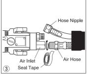
③Seal tape on the Air Hose Nipple and screw it in the Air Inlet on the tool.
