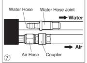
TSimilarly connect the Air Hose to the compressor, as shown in the illustration.
