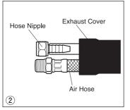
2 Insert the Hose Nipple into the Water Hose.
