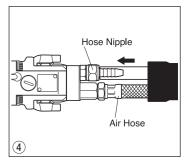
4 Put the Water Hose Nipple in the Water Inlet and fix it by the nut on the nipple.
