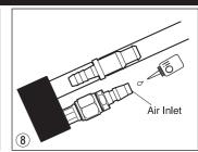
(8) Prior to operations, inject approx. 0.5cc (2 to 3 drops) air tool oil from the Air Inlet. And carry out the test run for 3 to 5 seconds, and allow air to circulate oil all over the tool.
