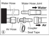
6Insert the Water Hose joint into the Water Hose, and connect it to the hose on the water faucet side, as shown in the illustration.
